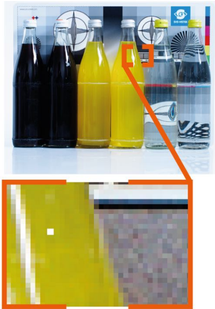
Fig. 5-22: Illustration of a defect pixel
