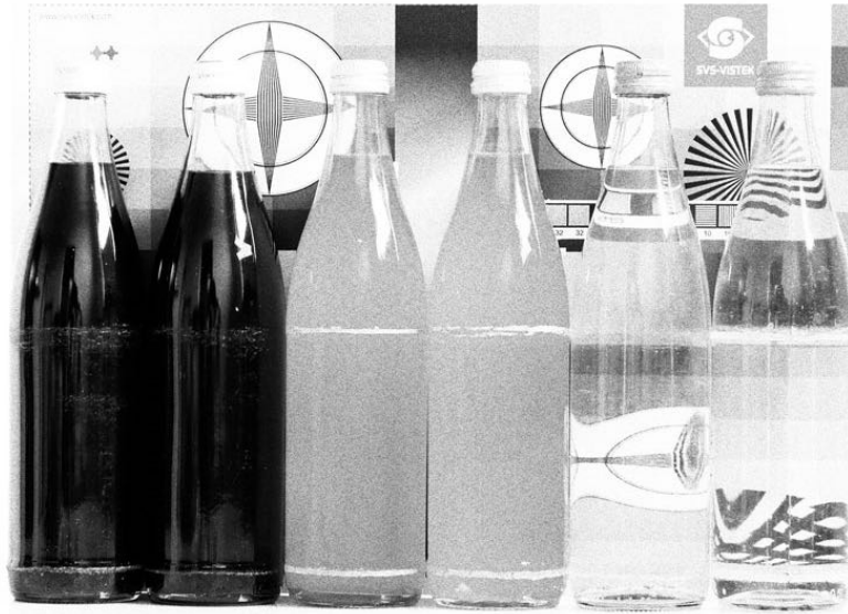
Fig. 5-1: Noise caused by too much gain
