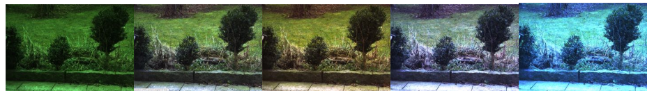
Fig. 5-36: Colour transformation OFF, D50, D65, TL84, A
