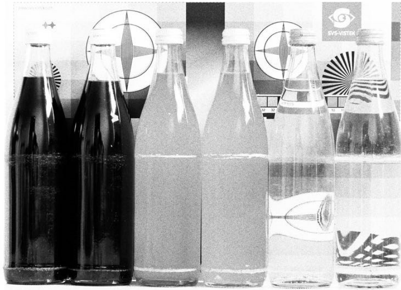
Fig. 5-1: Noise caused by too much gain
