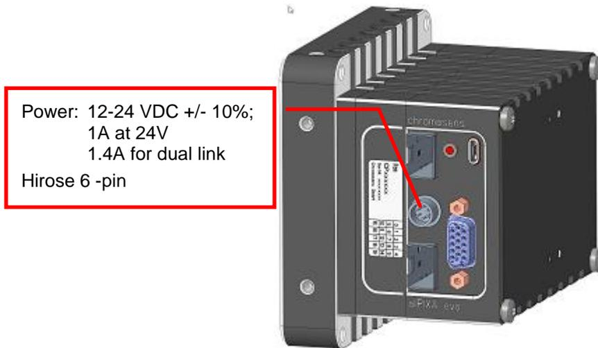
**Figure 22: Connecting the allPIXA evo camera to the power supply**
