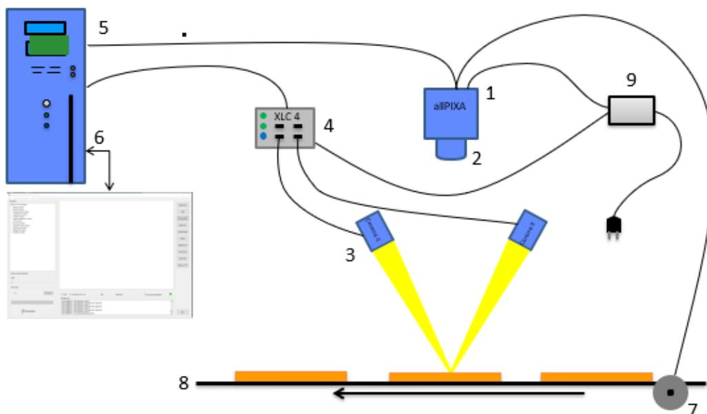
**Figure 1: Design of a line scan camera application**
