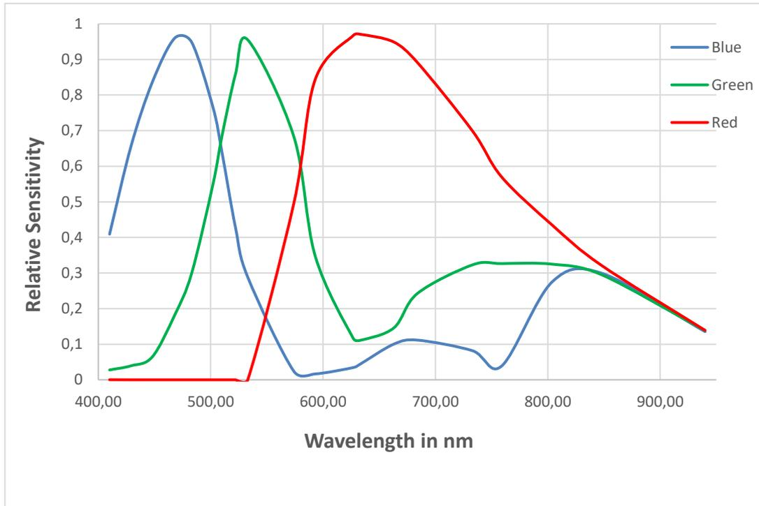
**Figure 5: Spectral sensitivity of the color camera line scan sensor**
