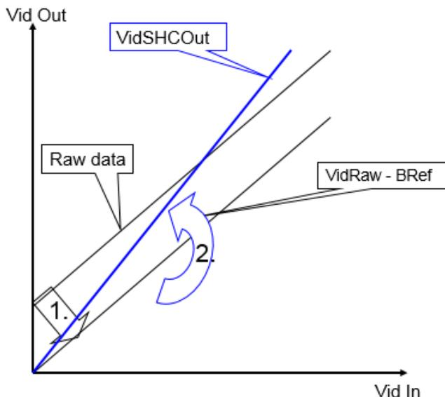
**Figure 11: Offset and shading correction**
