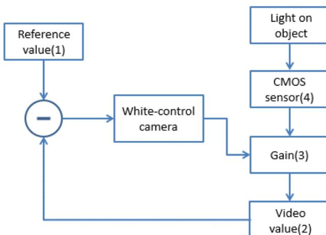
**Figure 12: Closed-loop control for white balancing**
