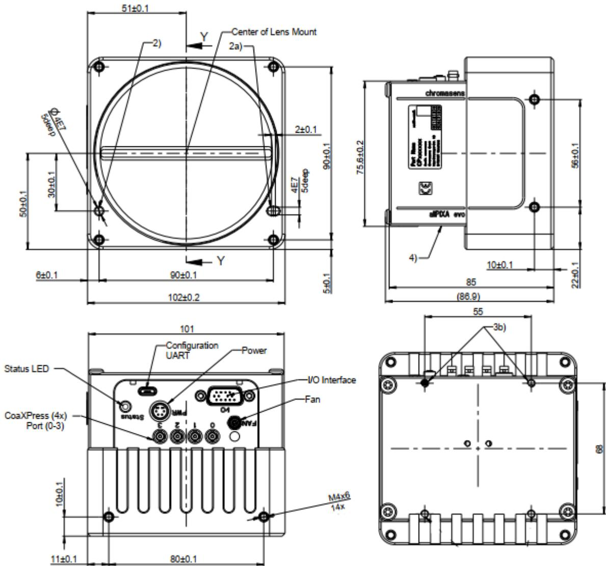
**Figure 32: allPIXA evo 15k camera (CoaXPress interface, Y variant)**
