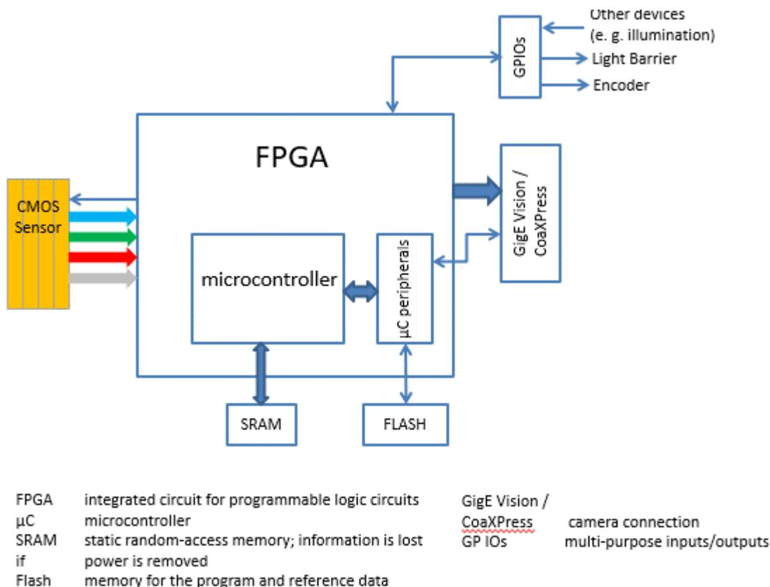
Figure 3: Basic design of the allPIXA evo camera (block diagram)
