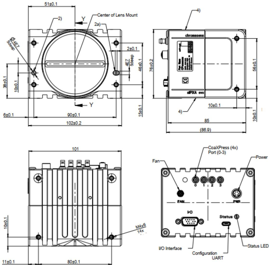
Figure 33: allPIXA evo 15k camera (CoaXPress interface, Z variant)
