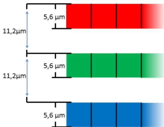
Sensor pixels are 5.6  $\mu\text{m}$  wide and 5.6  $\mu\text{m}$  long. The distance between the color sensor lines is 11.2  $\mu\text{m}$ .
