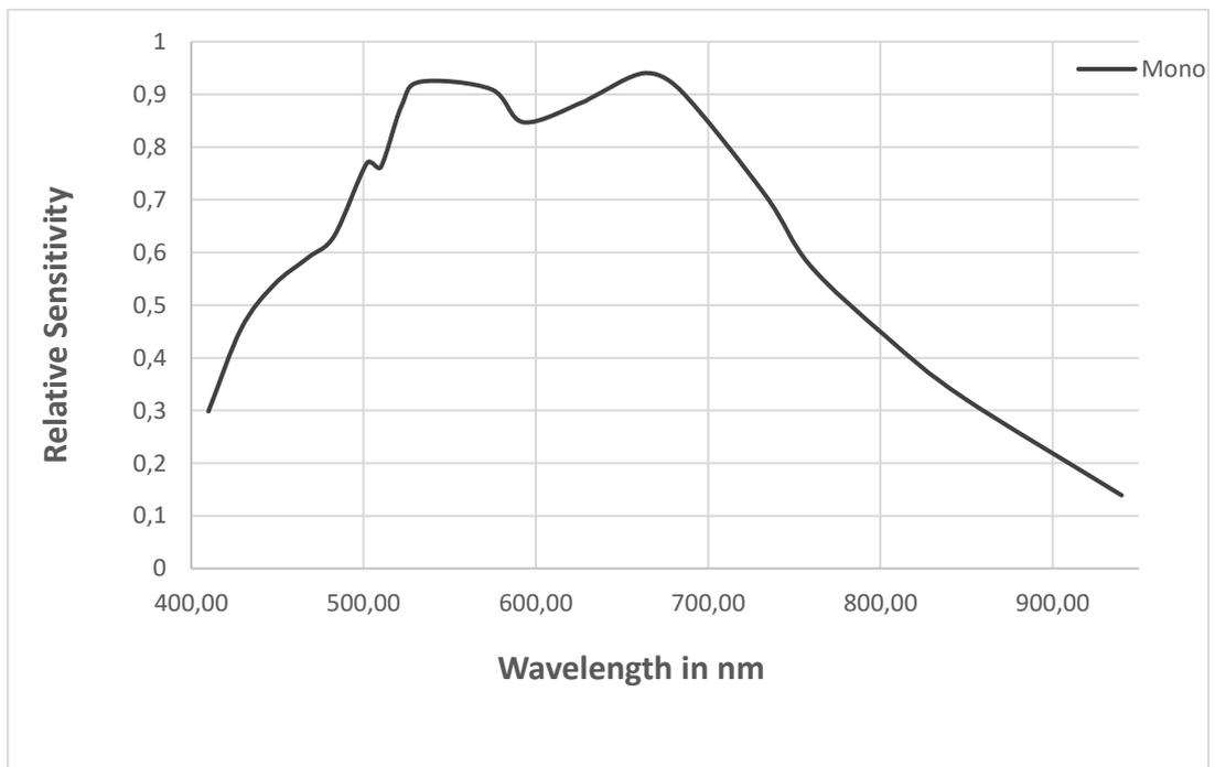
**Figure 6: Spectral sensitivity of the mono camera line scan sensor**
