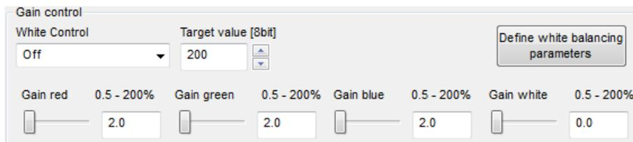
At the **White control** list, specify whether white control/balancing should operate continuously, only once per frame, or whether it should be switched off. If you select **Continuous**, the camera gain values are adjusted continuously during the scanning process.
