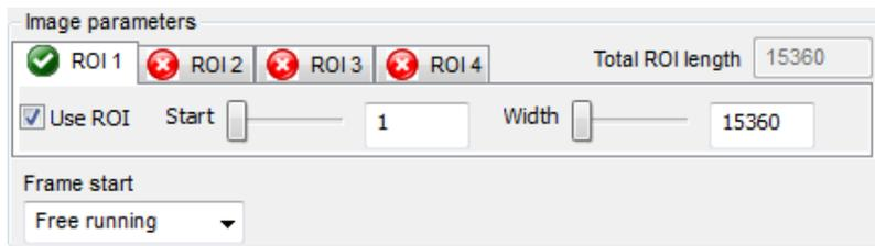
To enable an ROI, click the respective tab, select the **Use ROI** check box, and enter start position and width.
