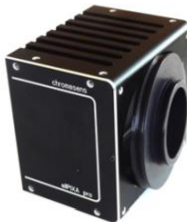
Figure 9: Mounting the lens adapter ring in the fit of the camera body
