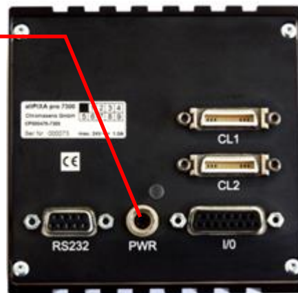
Figure 28: Connecting the allPIXA pro camera to the power supply
