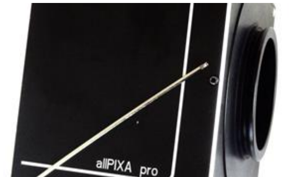
Figure 10: Securing the lens adapter ring to the camera
