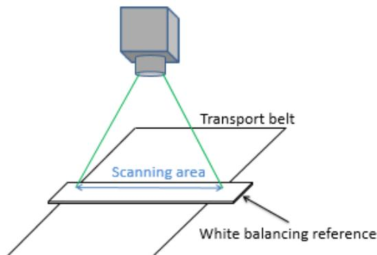
**Figure 32: allPIXA camera with a white balancing reference**
