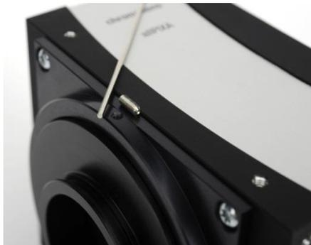
**Figure 25: Securing the lens adapter ring to the retrofit adapter**
