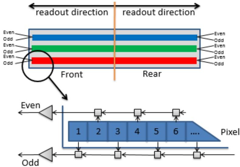
Figure 6: The allPIXA camera line scan sensor readout principle
