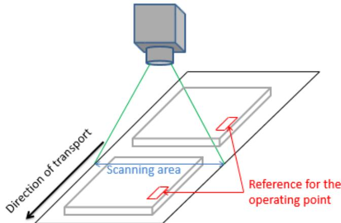
**Figure 34: Image-synchronous operating point adjustment on the object (ROI)**
