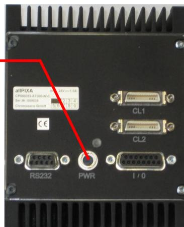
**Figure 32: Connecting the allPIXA camera to the power supply**
