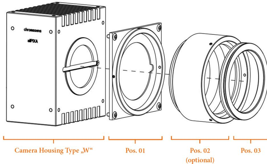
**Figure 19: configuration scheme (housing type W)**
