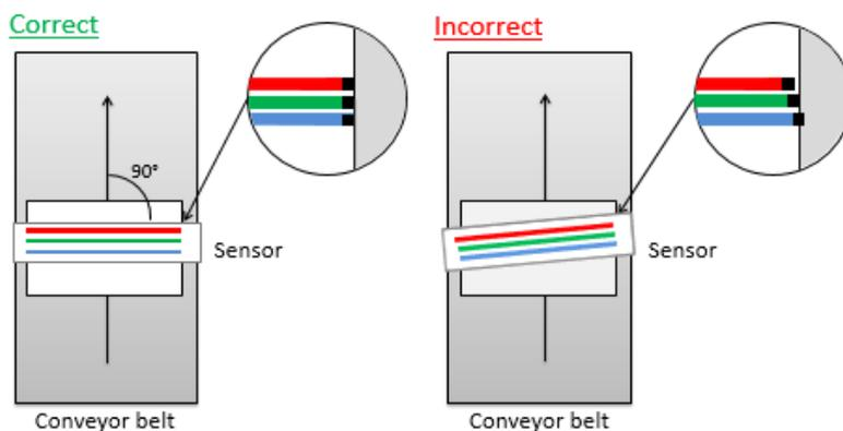
**Figure 28: Rectangularity of the sensor to the object**
