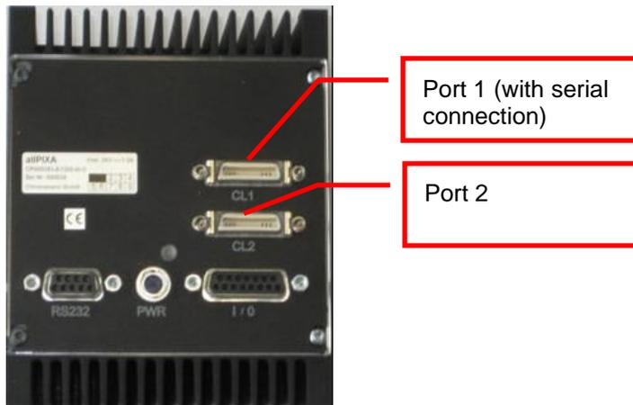
**Figure 1: Connecting the allPIXA camera to a PC**
