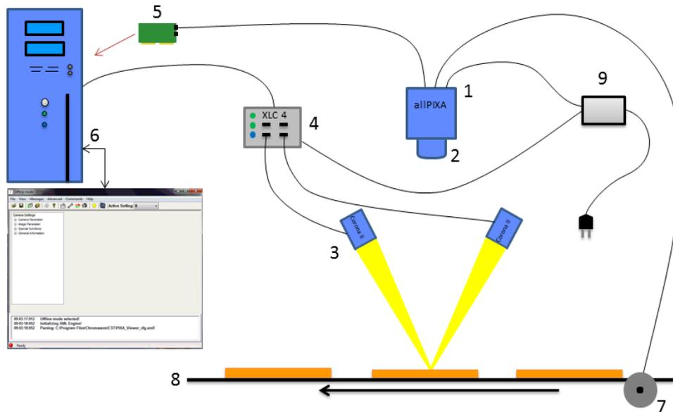
**Figure 1: Design of a line scan camera application**
