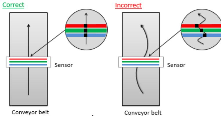
**Figure 27: Optimum conveying belt tracking**
