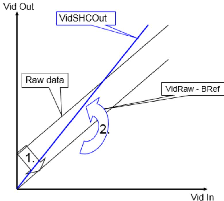
**Figure 14: Offset and shading correction**
