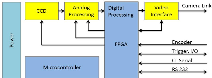
**Figure 8: Process of the allPIXA camera image processing (block diagram)**
