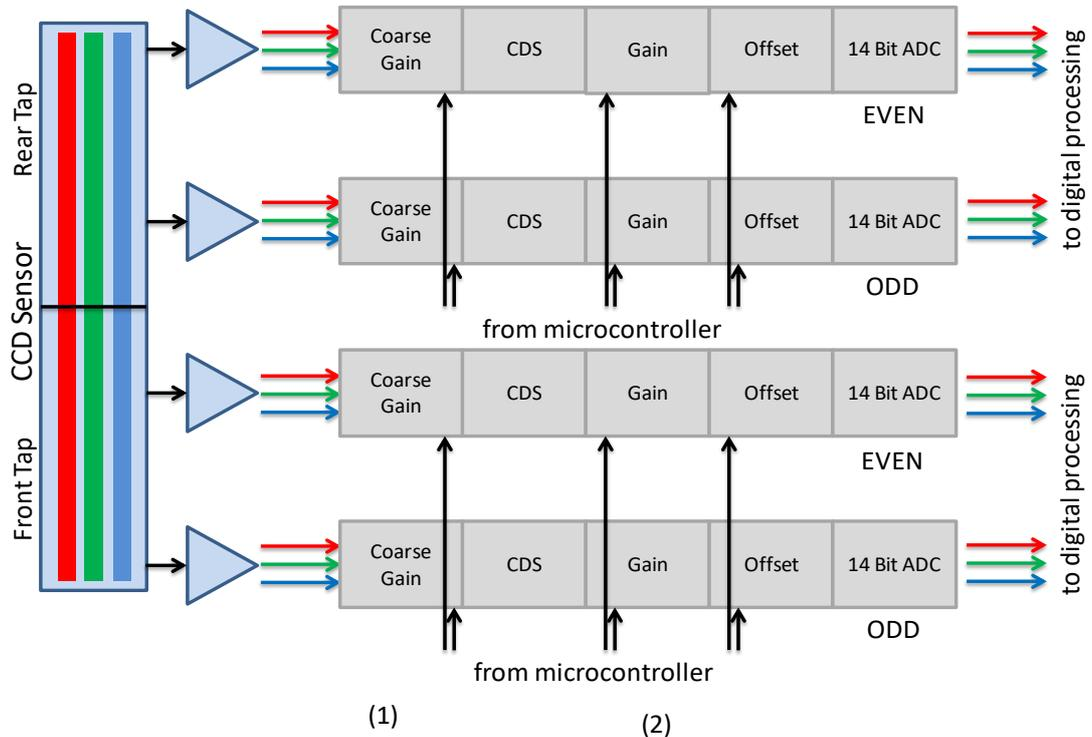
**Figure 9: Analog process of the allPIXA camera (block diagram)**
