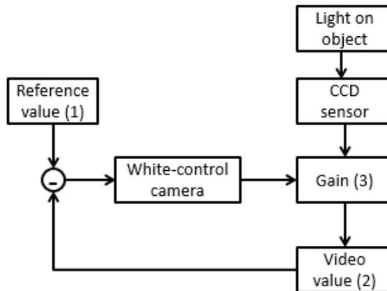
**Figure 15: Closed loop control for white balancing**
