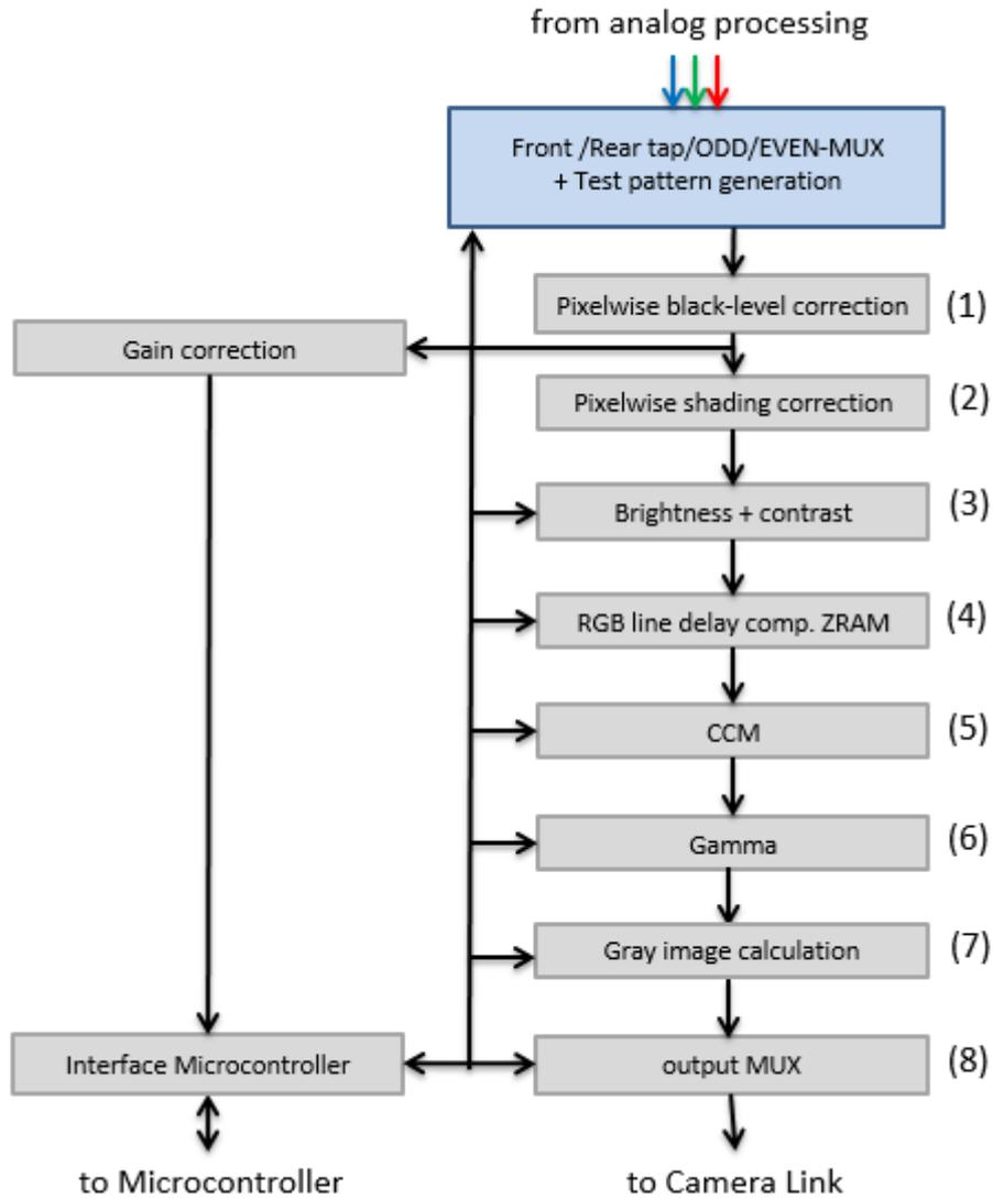
**Figure 10: Digital process of the allPIXA camera (block diagram)**
