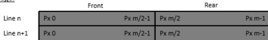
**Figure 11: Image information output on the CameraLink**
