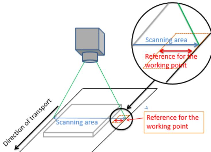
**Figure 33: allPIXA camera with continuous automatic white balancing**
