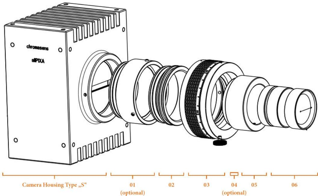
**Figure 20: configuration scheme (housing type S)**
