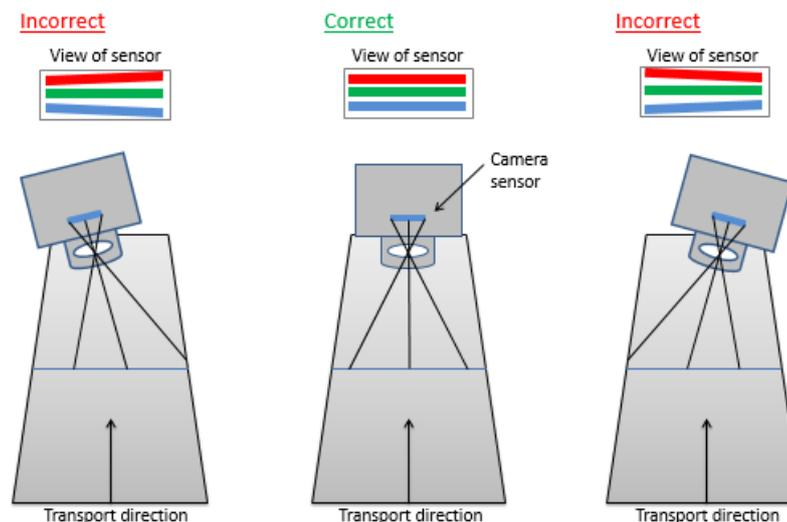
**Figure 30: Rotation around the transverse axis of the line scan sensor**
