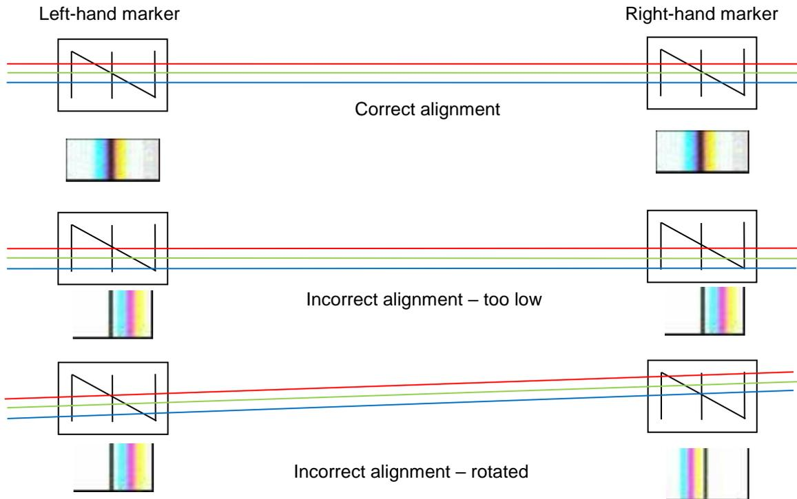
**Figure 31: Alignment of the allPIXA camera**
