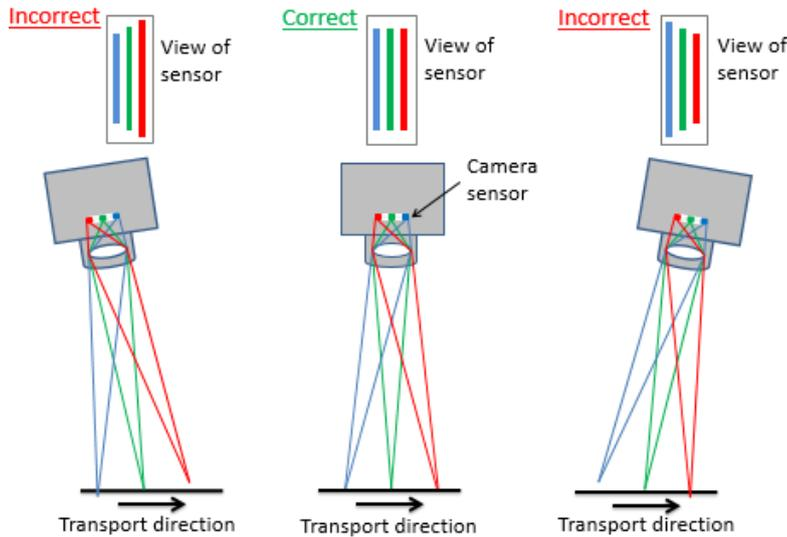
**Figure 29: Rotation around the longitudinal axis of the line sensor**
