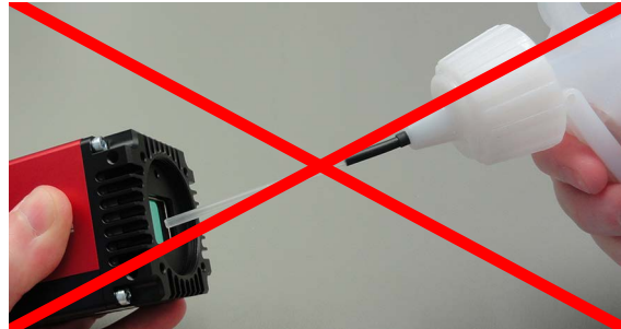
Figure 110: How not to use compressed air
