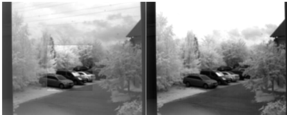
Figure 96: Left: auto contrast applied to ROI, right: auto contrast applied to the whole image.
