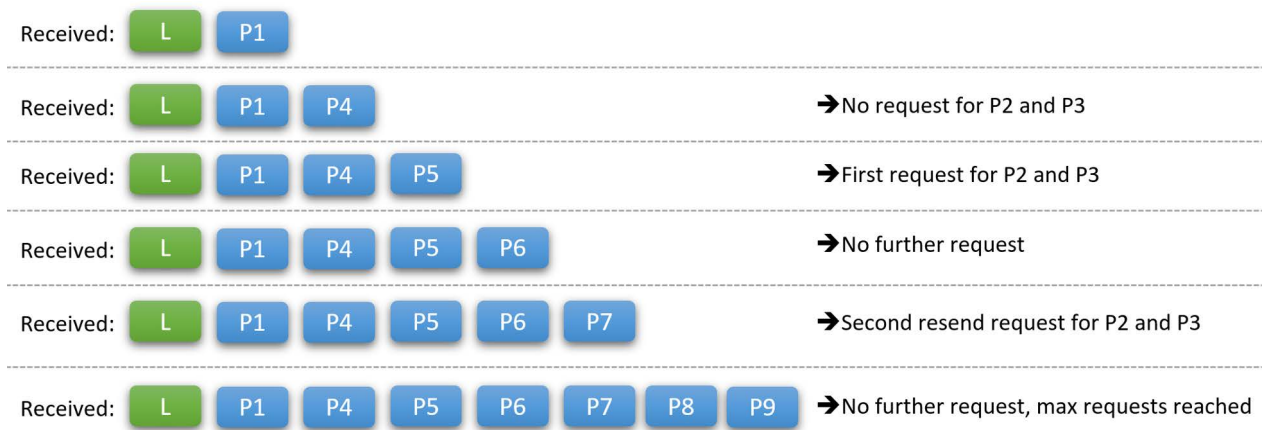
Figure 63: Controlling the resend of packets (example)
