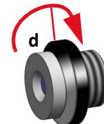
Figure 81: Lens and fixing nut
