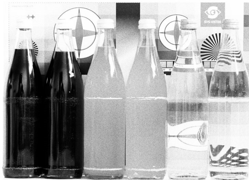
Fig.: 6-1: Noise caused by too much gain
