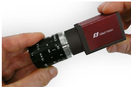
Figure 85: Illustration of camera orientation when removing lens or dust cap
