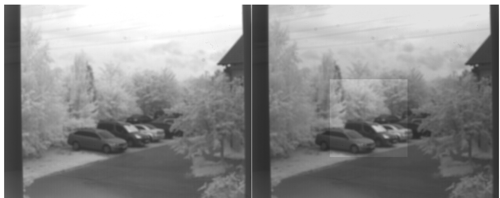
Figure 84: Example for the effect of AutoModeRegionDimOutside. Left: without dimming applied, right: with dimming applied to the outside area.
