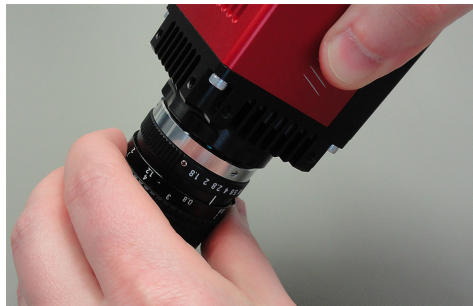
Figure 94: Illustration of camera orientation when removing lens or dust cap
