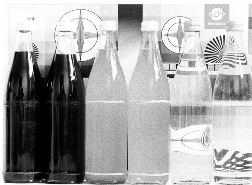
Fig.: 6-1: Noise caused by too much gain
