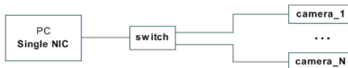
Fig.: 4-4: Illustration of connecting multiple cameras by a switch
