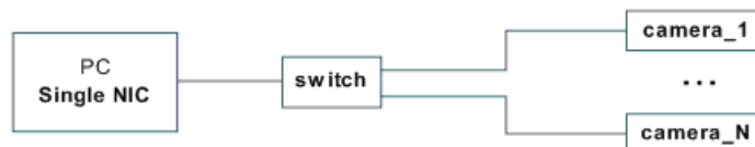
Fig.: 5-4: Illustration of connecting multiple cameras by a switch
