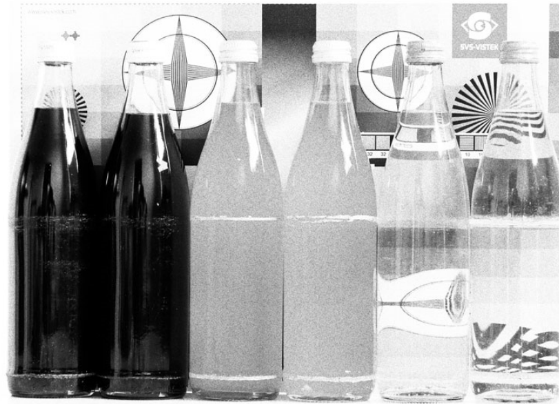
Fig.: 6-1: Noise caused by too much gain
