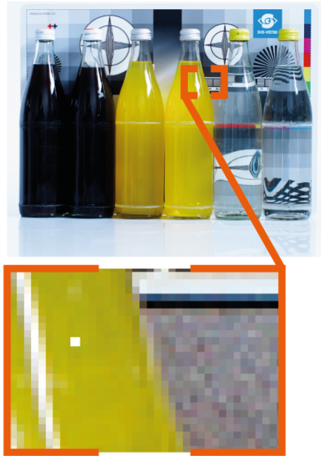
Fig.: 6-20: Illustration of a defect pixel
