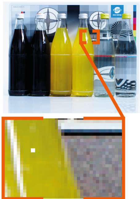
Fig.: 6-24: Illustration of a defect pixel
