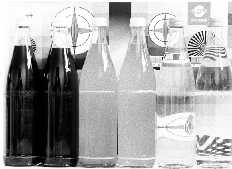
Fig.: 6-1: Noise caused by too much gain
