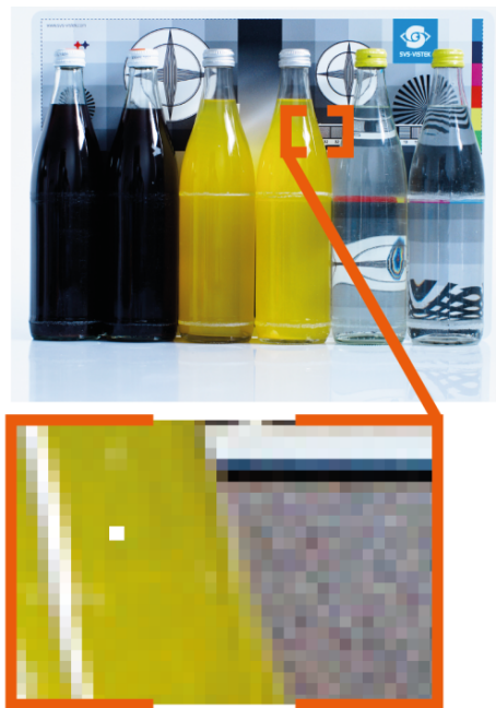
Fig.: 6-34: Illustration of a defect pixel
