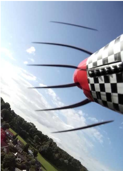
Figure 10: propeller w/ rolling shutter artifacts
