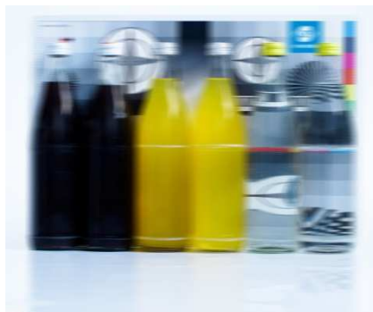
Figure 7: moving object, global shutter
