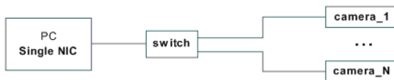
Figure 5: Illustration of connecting multiple cameras with a switch
