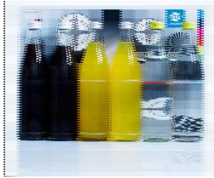
Figure 9: moving object, interlaced camera
