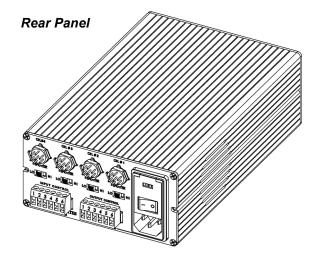
All main input/output functions can be accessed at the VMM-D3 rear panel, including the 115/230VAC input. Manual switching as required. Additionally, (2) 6-pin pluggable terminal strips allow for easy termination to input (active high) and output (active low) signals. Channel #4 is not operational.
