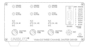
Simple and straightforward controls allow the VMM-D3 to be easy to use and configure. LED indicators reveal each shutter's status at a glance. Three fuse holders with .6A slow blow fuses, accessible at the front panel for ease or replacement. N.O./N.C. switches allow manual shutter operation. Addressable RS-232C control is available via the DB-9 connector. Address selected by SW1.
